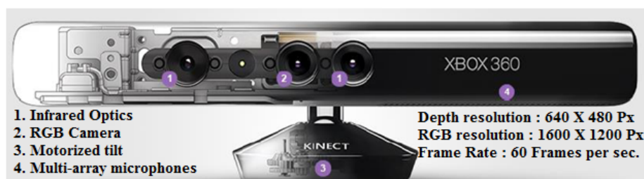
Fig. 11 Schematic diagram of the Kinect Sensor
