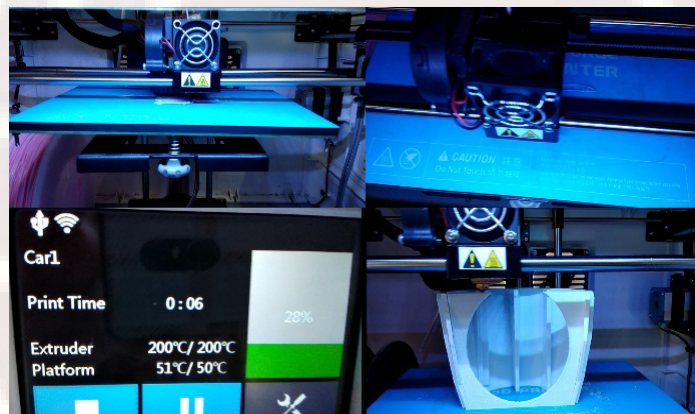
Fig. 2 Construction of different parts of the arm using a 3D Printer
